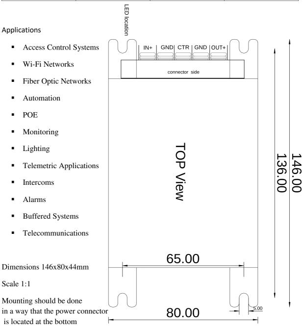
of the device, allowing for proper gravitational cooling.
